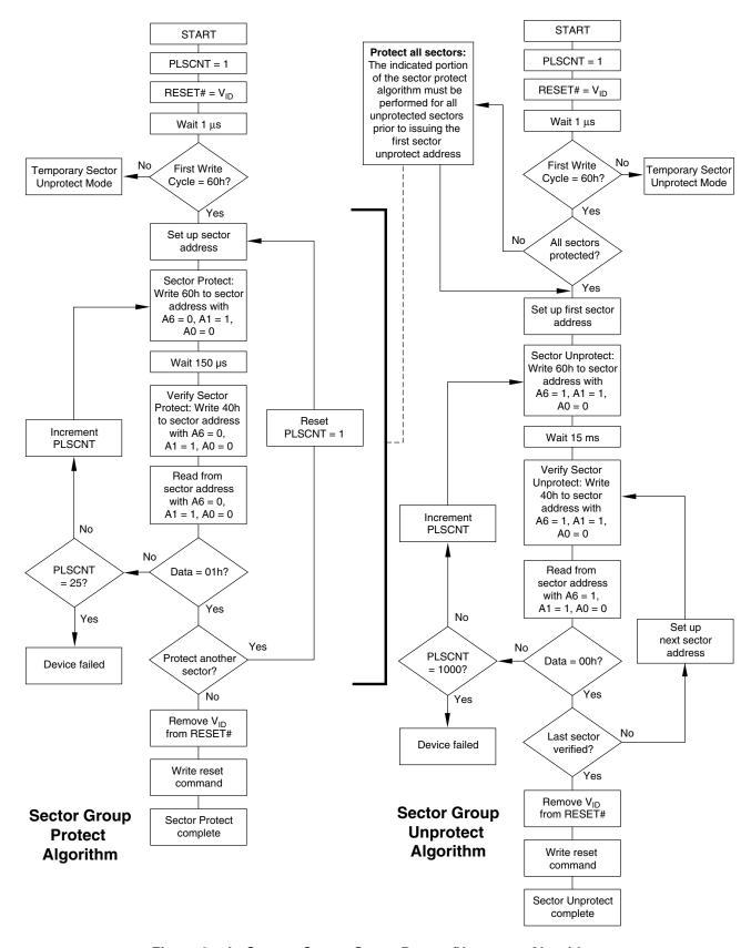
Figure 2. In-System Sector Group Protect/Unprotect Algorithms
