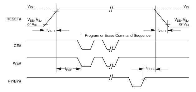
Figure 24. Temporary Sector Group Unprotect Timing Diagram
