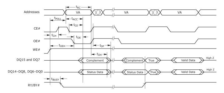
**Note:** VA = Valid address. Illustration shows first status cycle after command sequence, last status read cycle, and array data read cycle.
