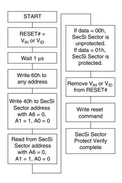
Figure 3. Secured Silicon Sector Protect Verify
