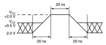
Figure 11. Maximum Positive Overshoot Waveform
