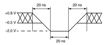
Figure 10. Maximum Negative Overshoot Waveform
