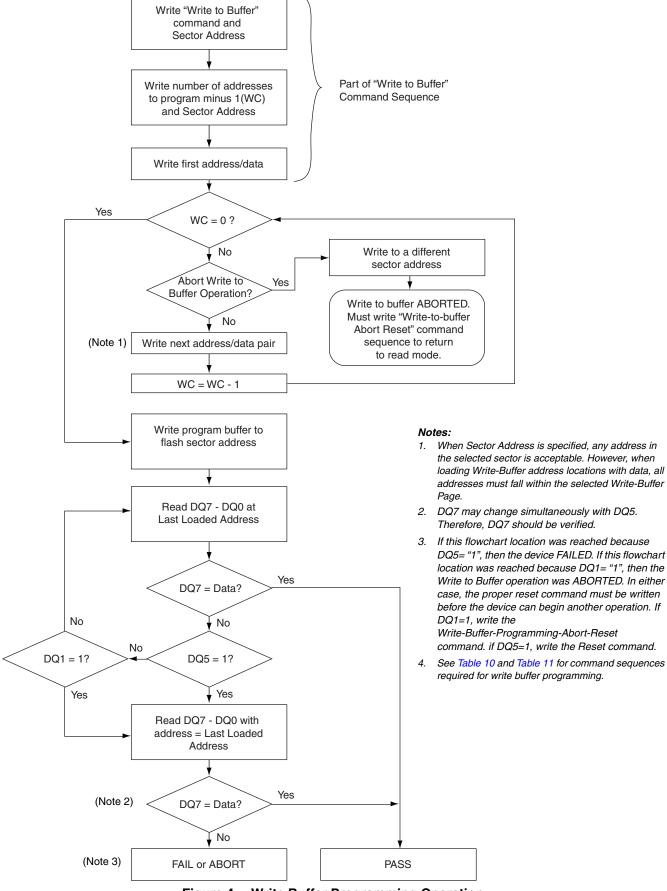
Figure 4. Write Buffer Programming Operation
